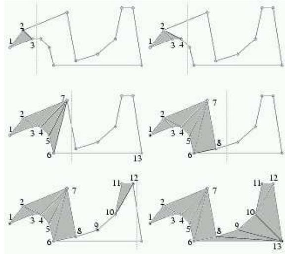
Figure 2: An example of triangulation around start points.<sup>2</sup>
