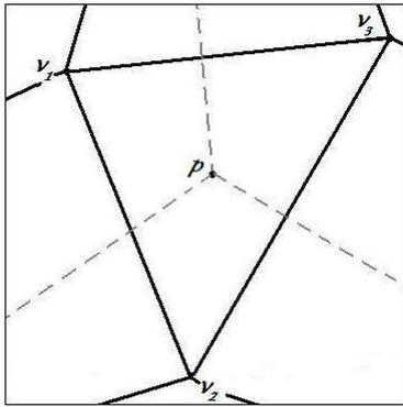
Figure 5: Solid, black lines indicate edges in  $DT(P)$ . Dashed, grey lines indicate edges in  $Vor(P)$ . The point  $p$  is a Voronoi vertex and is thus a candidate LEC center. Here,  $p$ 's three nearest neighbors are the three points contained in the Voronoi cells adjacent to  $p$ , which are the vertices of  $p$ 's dual triangle in  $DT$  space,  $v_1$ ,  $v_2$ , and  $v_3$ .
