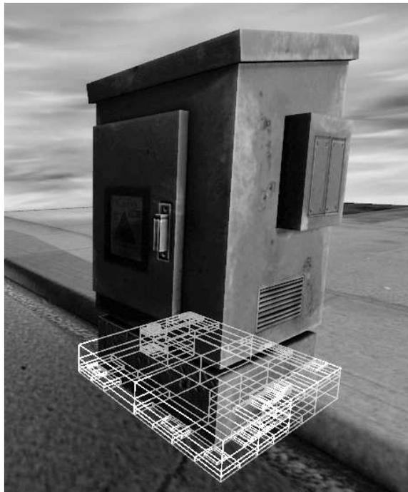
Figure 3: The intersection octree generated by a power transformer and a detailed sidewalk. The octree returned 70 pairs of triangles that might intersect, out of 846,000 possible pairs.
