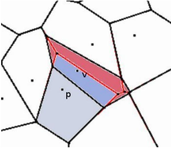
Figure 1: This figure shows the Voronoi cell for the inserted point  $v$  overlaid on the Voronoi diagram for the original point set. One of  $v$ 's natural neighbors,  $p$ , is shown with its Voronoi cell shaded. The area stolen by the insertion of  $v$  can be seen in the overlap between the two Voronoi cells.
