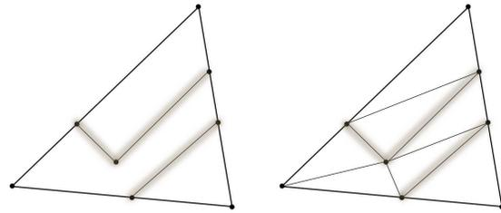
Figure 10: The constrained Delaunay triangulation (right) is guaranteed to preserve the lines of intersection (left).
