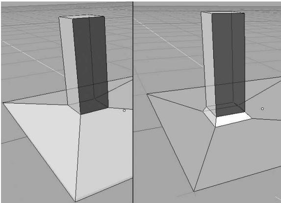
Figure 5: Without an auxiliary intersection (left), the deformation propagates in an uncontrolled way. With the auxiliary intersection (right), we have precise control over the shape of the deformation.
