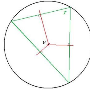
Figure 2: The circumcircle for a triangle  $T$ , whose center  $v$  is found by perpendicular bisector construction. If  $T$  is a triangle in a Delaunay triangulation, the  $v$  is the Voronoi vertex obtained when dualizing the Delaunay triangulation to the Voronoi diagram.
