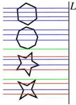
Figure 1: The top two polygons are monotone because every line only intersect the polygon twice.<sup>1</sup>
