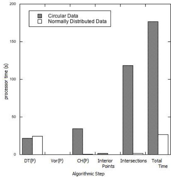
Figure 11: Processor time used by our algorithm on 1000 data points lying on a circle as compared to 1000 normally distributed, randomly generated data points.
