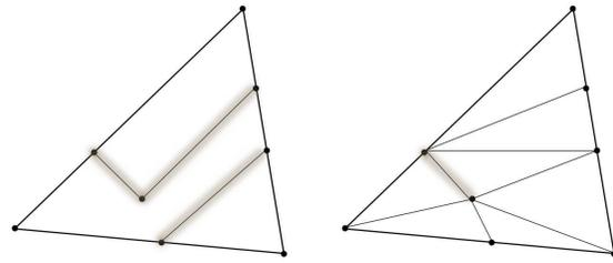
Figure 9: The Delaunay triangulation (right) does not necessarily preserve the lines of intersection (left).
