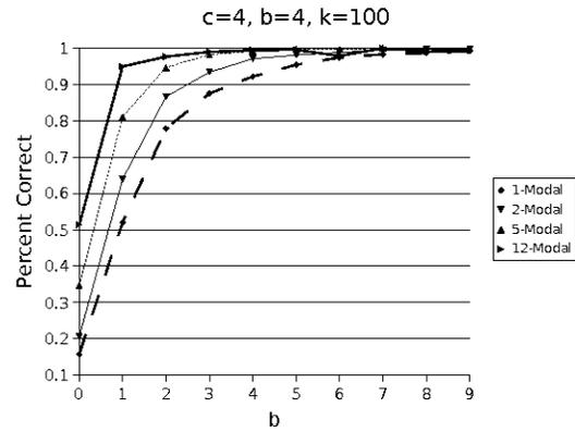
Figure 5: Algorithm 2 on synthetic data sets with 3000 points in 50 dimensions. For  $b > 4$ , nearly 100% of the nearest neighbors are correctly identified. Surprisingly, Algorithm 2 does better on more complicated distributions.
