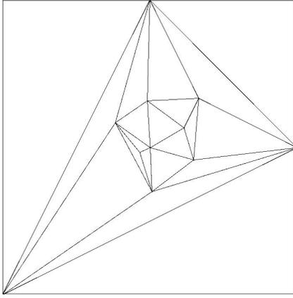
Figure 1: A simple example of the Delaunay triangulation computed on a small set of points.
