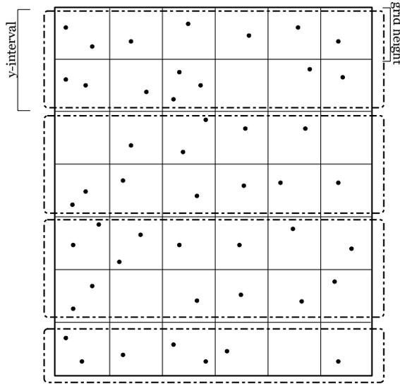
Figure 1: Splitting the grid into sub-grids for parallelization
