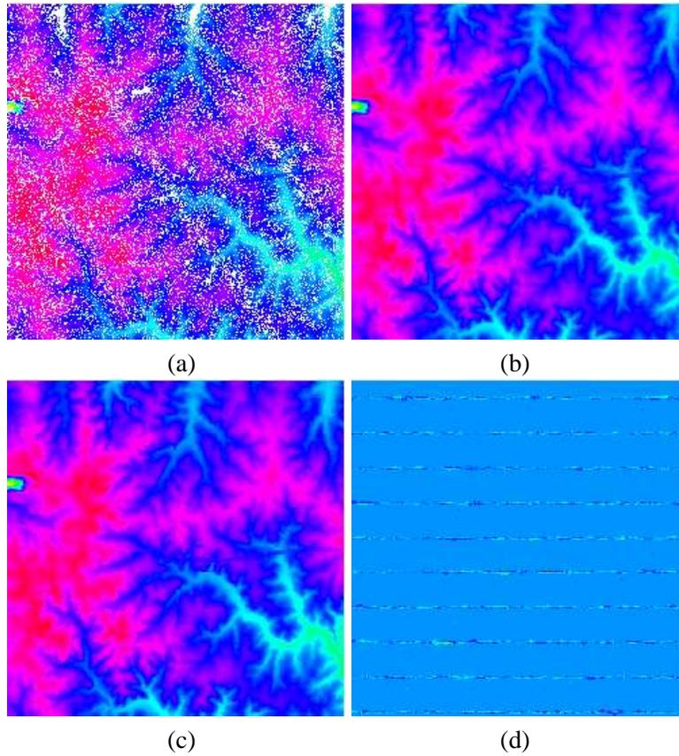
Figure 2: Results of interpolating sparse data at 100 feet. (a) is the result of binning - note the cells with no value. (b) is our parallel interpolation algorithm without smoothing, and (c) is with smoothing. (d) is the difference between (b) and (c).
