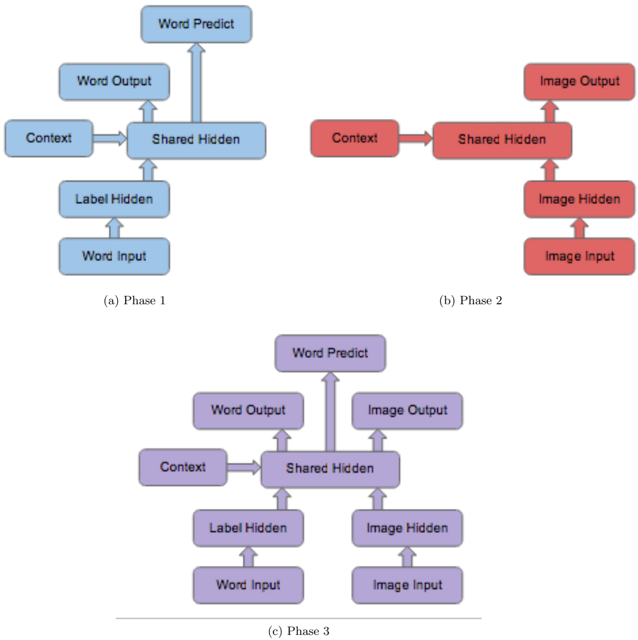
Figure 4: Active layers during the each phase. Only these layers feed activation forward or have their weights changed by backpropagation.
