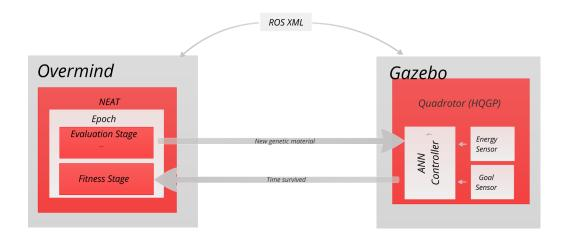
Figure 3: This diagram shows the architecture of HERP and our neural network test harness, Overmind.
