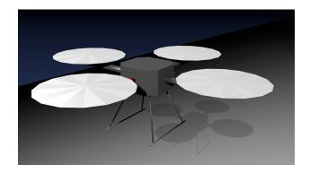
Figure 2: This is the quadcopter model provided by hector\_quadrotor for simulation in Gazebo, dubbed "HERP" for the purposes of these experiments. Rendering from [5].
