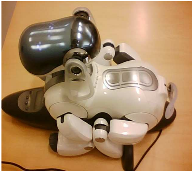
Figure 2: Buttons on the Aibo's back were used to administer reward and punishment.
