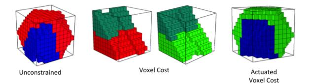
Figure 3: Characteristic phenotypes for traditional NEAT evolved softbots. Red is phase1 muscle, light green is phase2 muscle, blue is hard passive, and dark green is soft passive.
