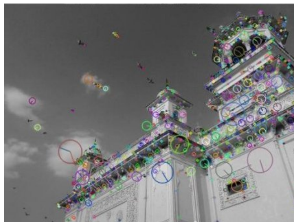
Figure 2. A picture of SIFT feature keypoints from OpenCV.
