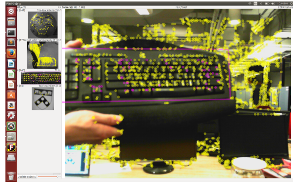
Figure 7. Image of using Find-Object-2D to extract keyboard features.
