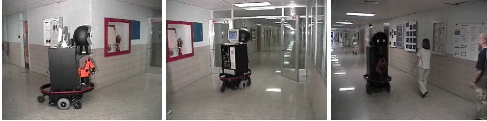
Figure 9: SAIL robot navigates autonomously using its autonomously developed visual perceptual behaviors. Four movies are available at http://www.egr.msu.edu/mars/ to provide more results.
