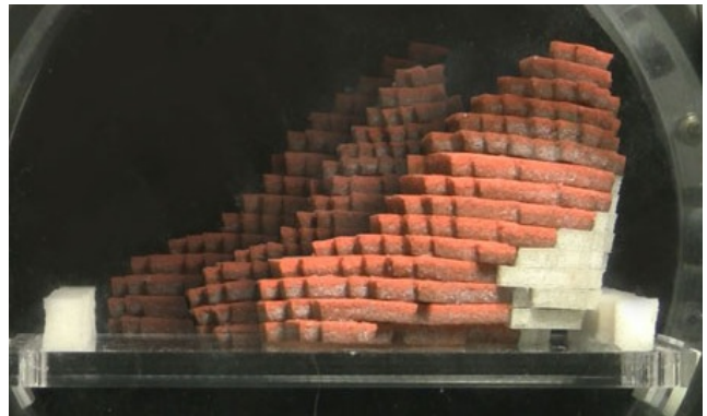
Figure 4: A time-series example of a fabricated soft robot, which actuates with cyclic 20% volumetric actuation in a pressure chamber [13]. This proof-of-concept shows that evolved, soft-bodied robots can be physically realized. Current work is investigating soft robot actuation outside of a pressure chamber.
